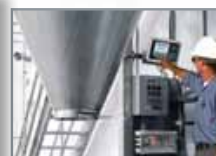
A 32-channel display capability allows viewing of weight on an individual scale and a combination of totalized scales.
