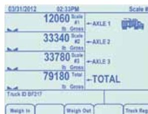
A 32-channel display capability allows viewing of weight on an individual scale and a combination of totalized scales.
